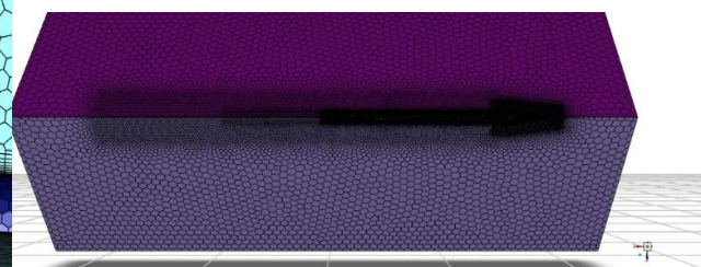
MESH GENERATION – UPPER ROCKET BODY
