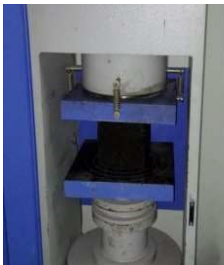
Figure3.Compressive strength test of cube using CTP
